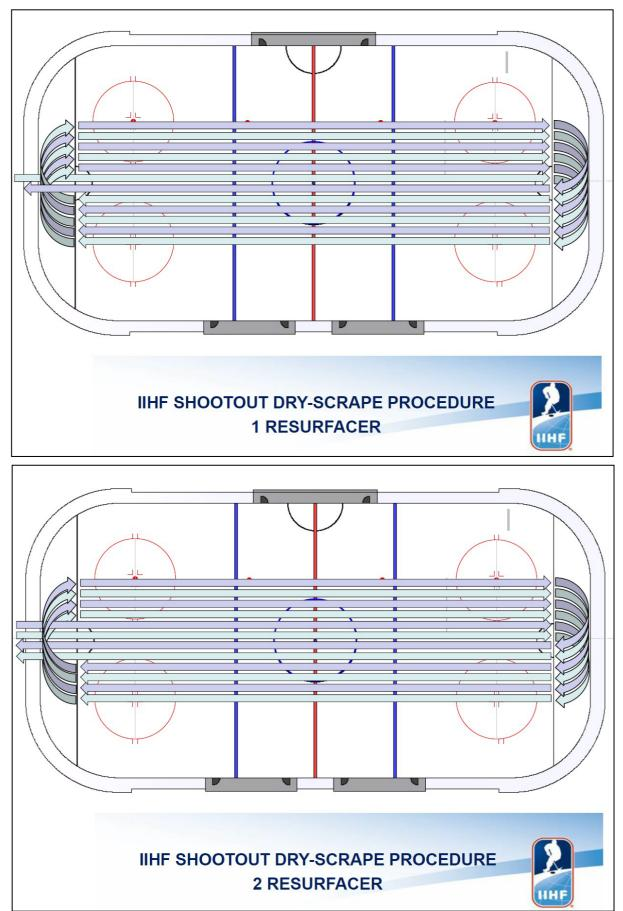
• The machine will continue this pattern (6 full laps) until the ice surface has been completely scraped between the face off spots (See diagram).
